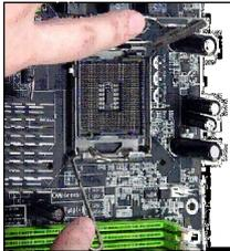
8. Correctly align the triangle of CPU Clip with the CPU chamfer, and the square on the CPU Clip to the hook of the socket.
