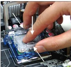
10. The CPU is installed well on the CPU socket.
