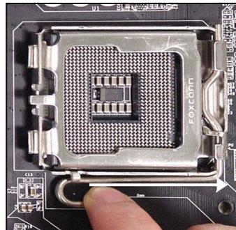
5. Lift the load lever up and open the load plate.
