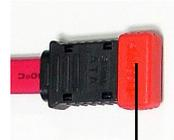
Take out the dust cover and connect to the hard disk devices
