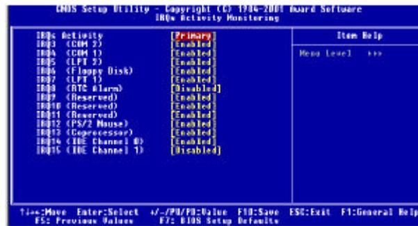
IRQ3 ~ IRQ15 enable or disable the monitoring of the specified IRQ line. If set to [Enabled], the activity of the specified IRQ line will prevent the system from entering power saving modes or awaken it from power saving modes.
